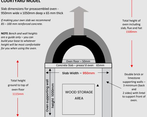
Footings approx. 100mm thick reinforced concrete
